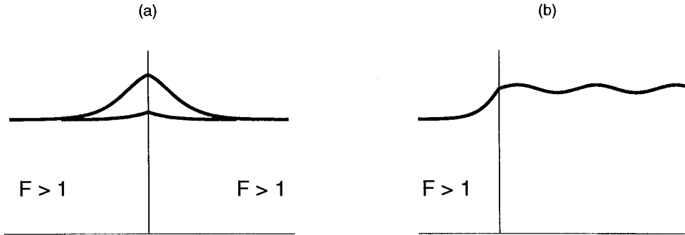
Figure 5. (a) Upstream supercritical flow. The forcing can sustain two symmetric solitary waves. (b) Solution matching the upstream supercritical flow with a cnoidal wave downstream. All these solutions lie in the region called ‘two solitary waves + infinity of wavy solutions’ in Figure 3.
